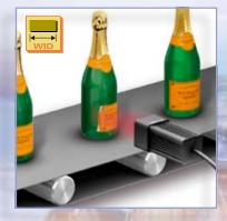
Width inspection The Width tool measures an object, in this case a label, to verify that it is not folded or cut.
