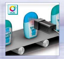
Hue verification The Hue tool inspects colour differences in a plain colour work-piece. A false colour cap will be rejected.
